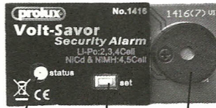
State ( warning ) light signal Mode setting button Buzzer
